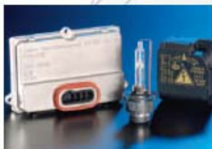
Mark 4 ballast with a xenon bulb.
