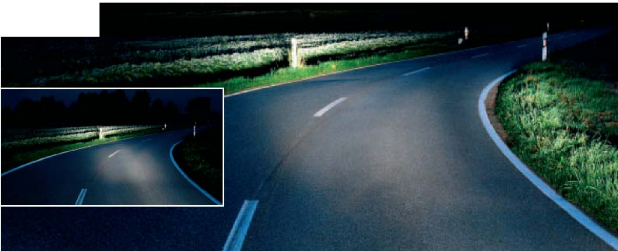
Conventional main beam light: the bend remains in darkness.
